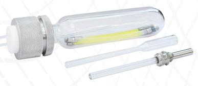
In a Trace Source™ Permeation Tube component compound contacts one side of a Teflon® membrane. Compound vapor slowly passes through the Teflon®. This vapor 'leak' is the emission rate of the permeation tube and is far too low flow to be controlled by conventional means.
