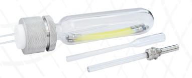
In a Trace Source™ Permeation Tube component compound contacts one side of a Teflon® membrane. Compound vapor slowly passes through the Teflon®. This vapor 'leak' is the emission rate of the permeation tube and is far too low flow to be controlled by conventional means.
